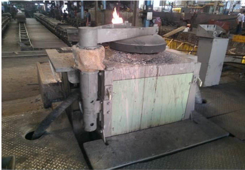
Lid mechanism for induction furnace crucible
